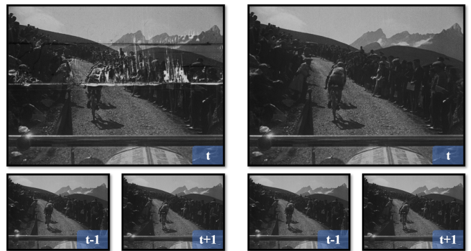
(a) Three consecutive frames with line scratches and blotches in the central one
