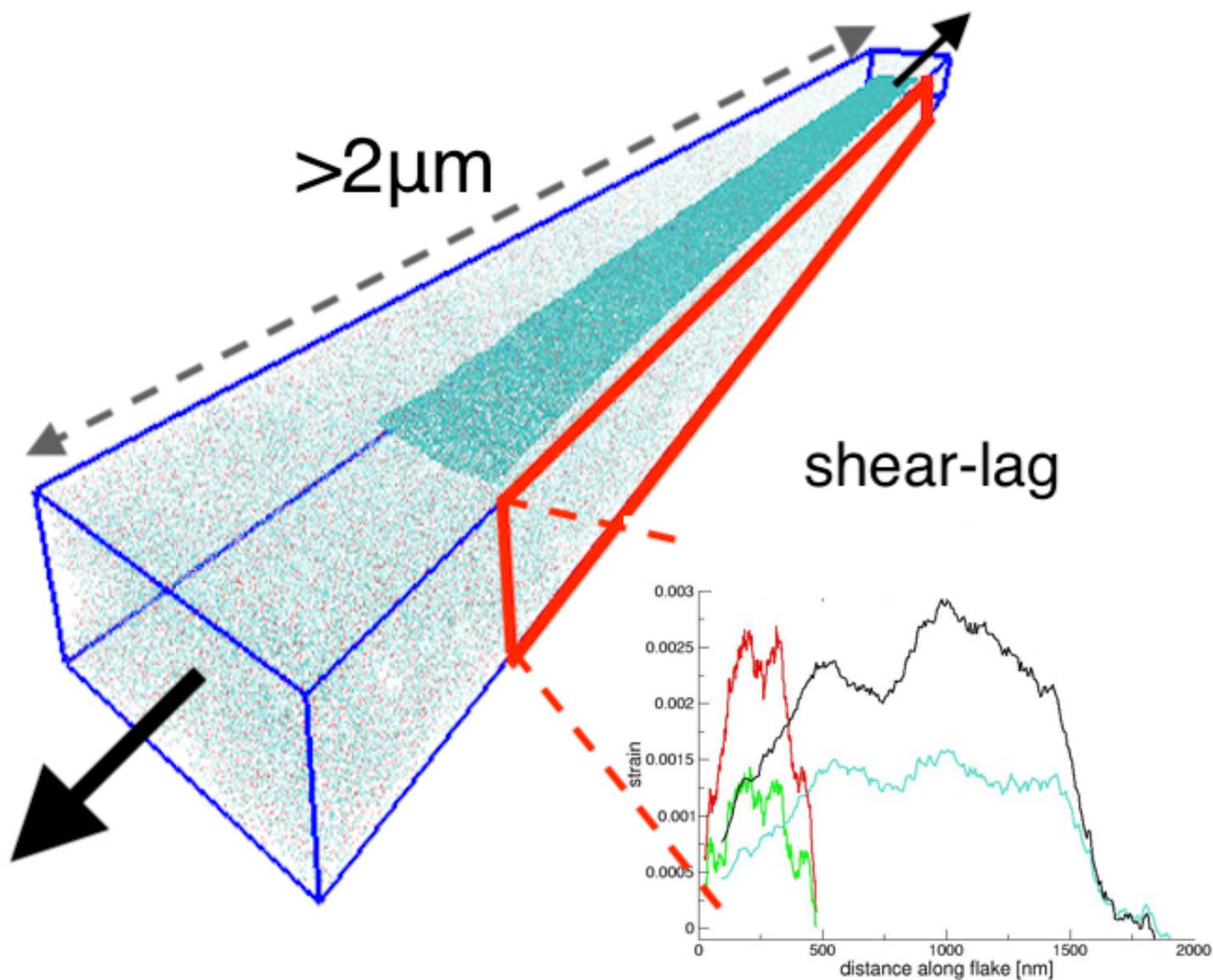
The mechanism of reinforcement of polymer materials by graphene-based inclusions is highly important for the design of high-performance composites. Very large molecular simulations show that graphene flakes can effectively reinforce the polymer matrix via a shear-lag process down to flake sizes of 500nm, as long as the flake is predominantly flat. However, even small undulations of the surface substantially degrade the enhancement of materials properties.
