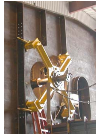
PHOTO 12: Portable Web Milling Machine
