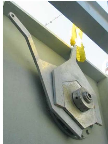
It is preferable to initially set the eccentrics or wedge assemblies in the shop in their centered position so as to maximize the PHOTO 13: Overhung Trunnion Eccentric
