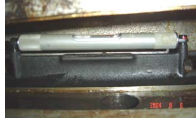
PHOTO 15: Trunnion Bearing Machinist Level Measurement
