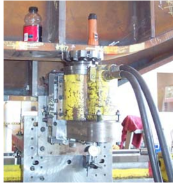
PHOTO 19: Flange Milling Operations
