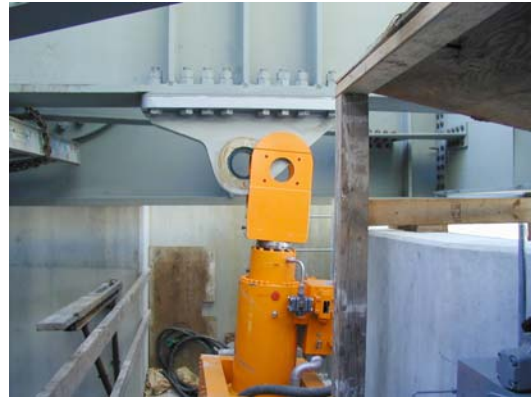
PHOTO 22: Hydraulic Cylinder Upper Clevis
