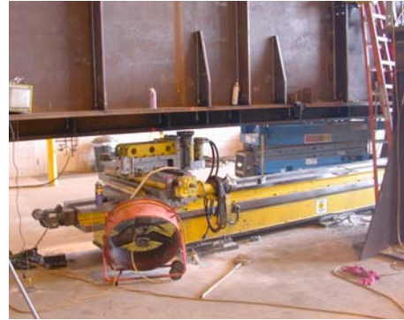
PHOTO 20: Portable Milling Table
