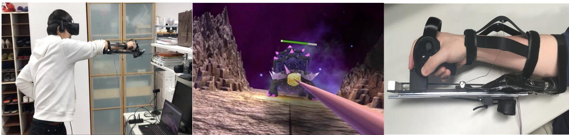
Figure 1: (Left) Player wears the HMD (head-mounted display) and our arm stretch device during gameplay. (Middle) The gaming screenshot in the HMD. (Right) Arm stretch device attached to player's forearm.
