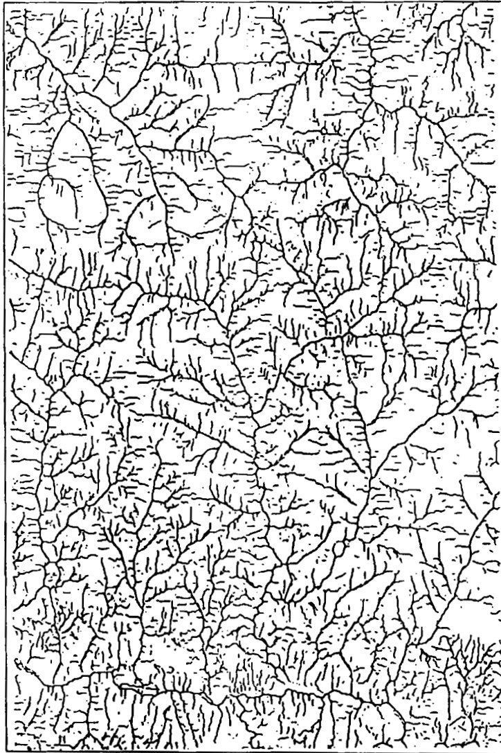
Figure 10. Pixels identified by the Peuker and Douglas Algorithm applied to the CALD dataset
