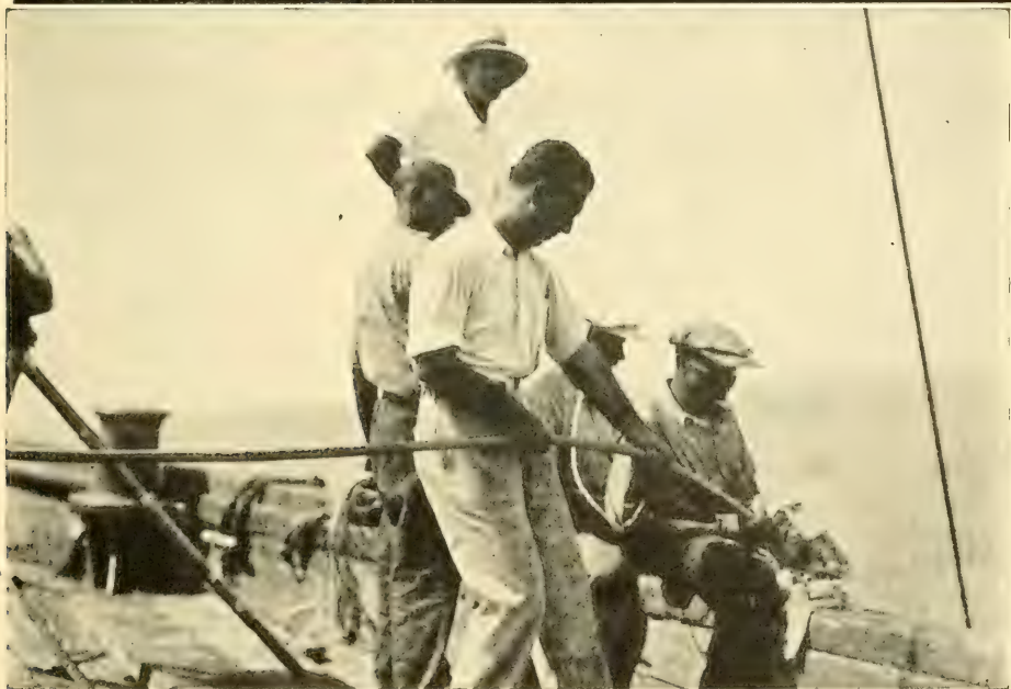
FIG. 92. ( upper ) A laboratory photograph of a viperfish ( Chauliodus ), of which I saw, from the bathysphere, a school of seven at a depth of 1700 feet. FIG. 93. ( lower ) The most delicate part of the operation of the descent is the paying out of the solid rubber hose containing telephone and electric light wires. This must not be bent or rubbed, and every 100 feet is fastened to the wire cable with a rope tie.
