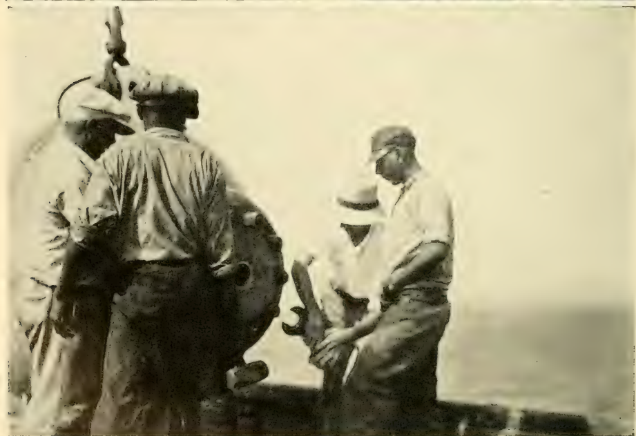
FIG. 67. ( upper ) The half-mile of solid rubber hose has now been unwound from its spindle and coiled loosely on deck. One weak spot has been cleverly spliced by a friend from the Wireless Station, and the four internal wires work perfectly, transmitting sound and light. A squall is approaching, making diving impossible, and the bathysphere is being lashed to keep it from rolling about. FIG. 68. ( lower ) Before a human goes down in the bathysphere it must be sent for a test dive, deeper than the intended descent. The 400-pound door is swung into place and fastened on.
