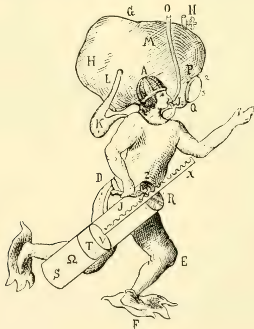
FIG. 10. This apparatus, impractical though it obviously was, contained the germ of the idea upon which modern diving suits are based—the removal of the confined air and the substitution of fresh. It was designed by Borelli in the seventeenth century.
