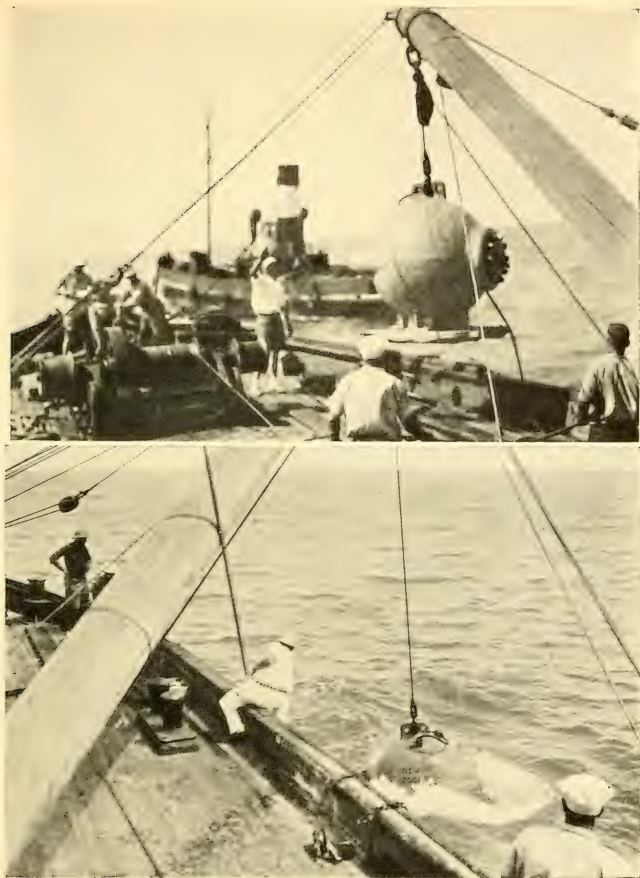
FIG. 69. ( upper ) The signal given, the great hollow mass of steel is lifted into the air and overboard. A large tug, the Powerful , is seen, standing by in case our boat should again spring a leak. FIG. 70. ( lower ) After being lowered to 3000 feet, the bathysphere is brought up again. One hundred feet from the surface it becomes visible. When lifted into the air, the creaking and straining of the machinery shows that something is wrong; the sphere is twice as heavy as it should be.
