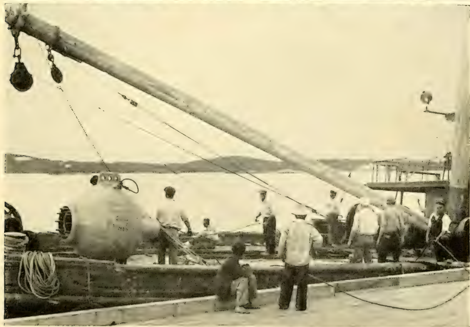
FIG. 61. ( upper ) We are now at the wharf where the bathysphere, winches and miles of cable have lain in their housing for a year and a half. The 3000-foot rubber hose, enclosing the telephone and electric light wires, is just coming aboard. FIG. 62. ( lower ) We see the bathysphere on the deck of the Freedom , and the enormous yard, brought especially from last year's boat. The low bulwarks and wide expanse of deck make this craft ideal for our work. But she proves to be anything but sea-worthy.
