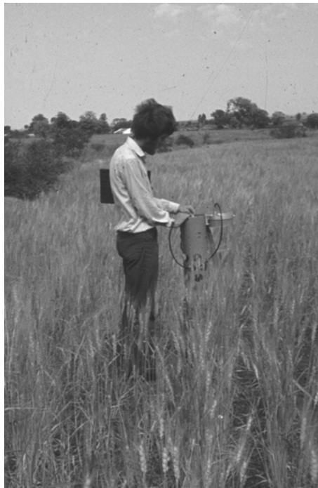
Plate 5.1 Neutron probe soil moisture measurement in the Nion basin.
