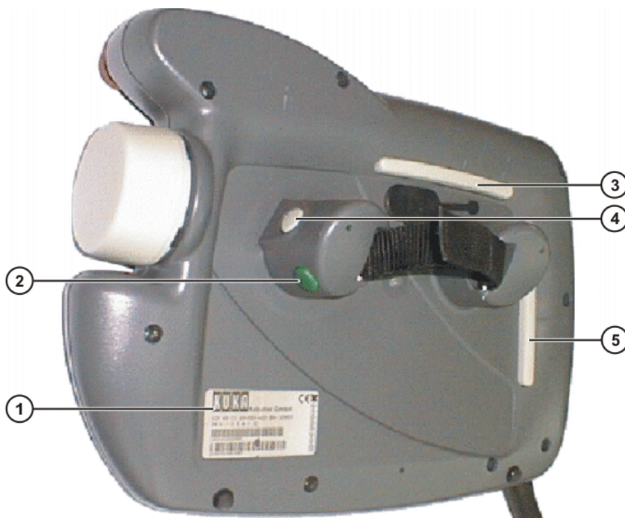
Fig. 2-11: Rear view of KCP
