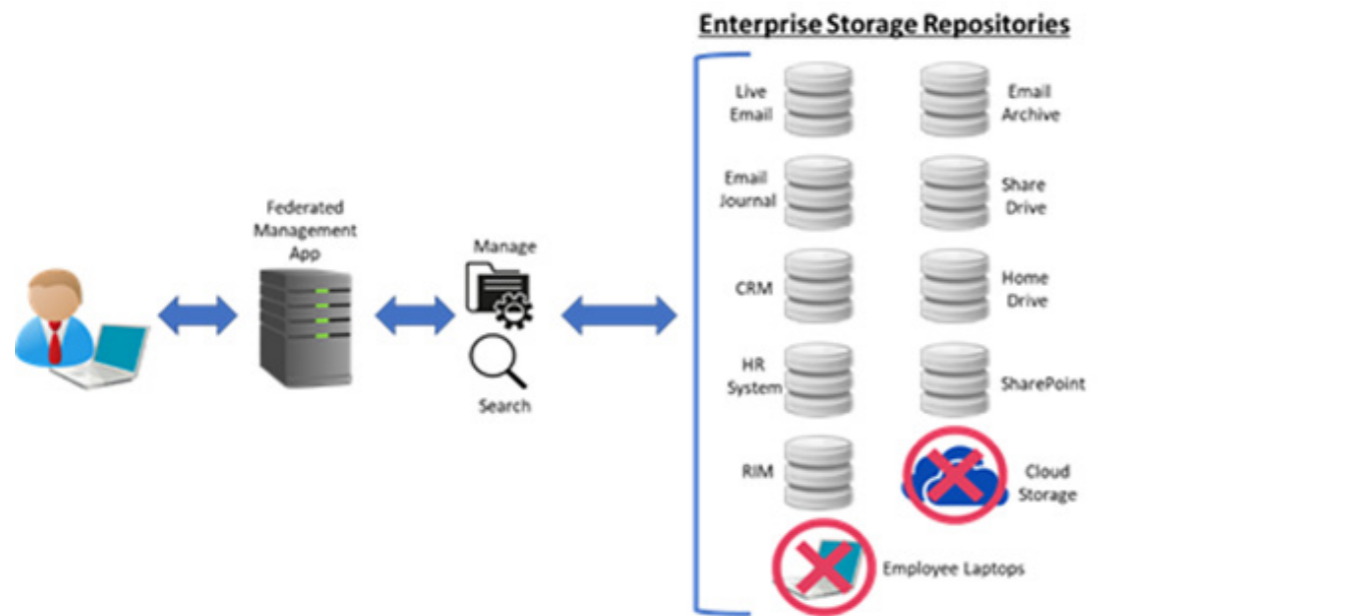
Figure 1: Federated Information Management manages files via policies from a centralized dashboard. This allows centralized search of all connected repositories.
