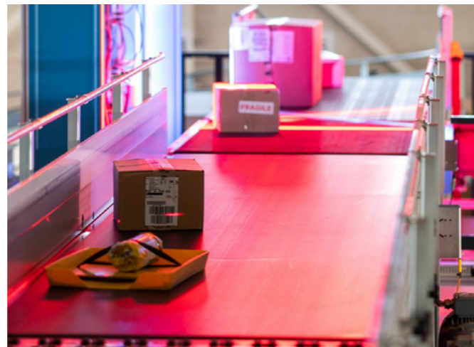
Text Vision operates by taking pictures of labels, enhancing them and then reconstructing the image using logic.
