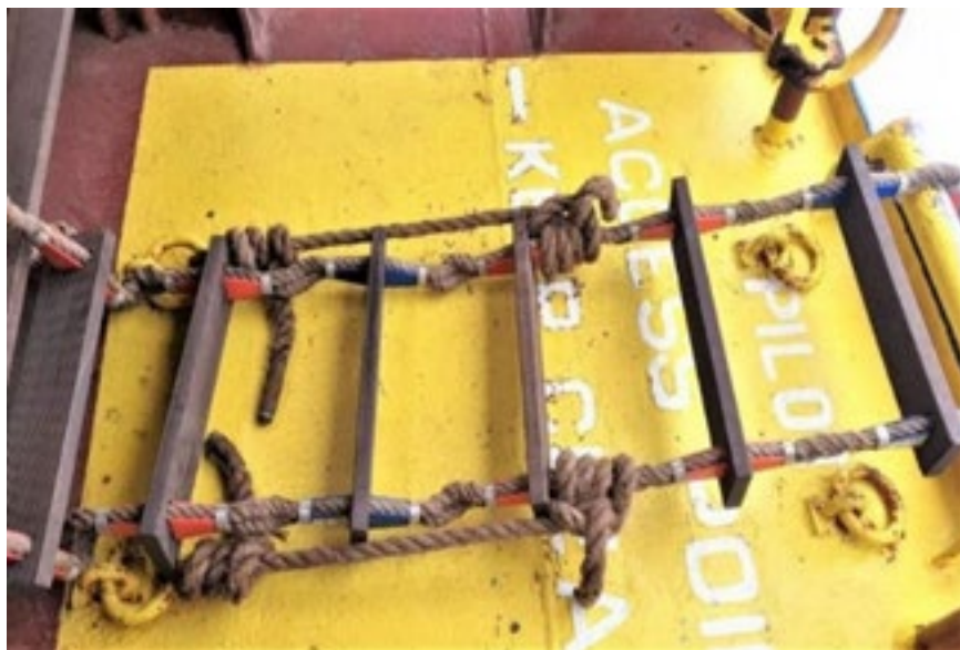
Photo 7: Rolling hitch knots being used to secure pilot ladders to approved main deck strong points (Reproduced with permission from Fremantle Ports). Photo credit: AMSA
