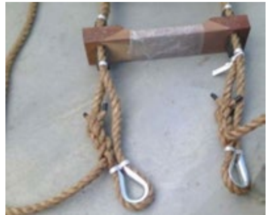
Photo 12: Example of non-compliant pilot ladder with splices inside ropes. / Credit: AMSA
