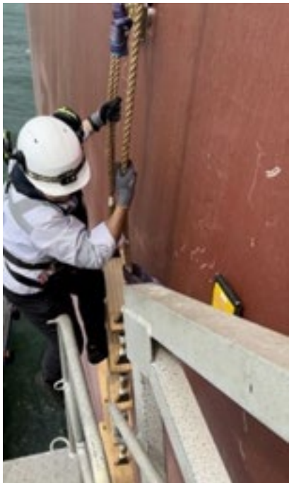
Photo 3: Person unable to safely access accommodation ladder platform from pilot ladder. Photo credit: AMSA
