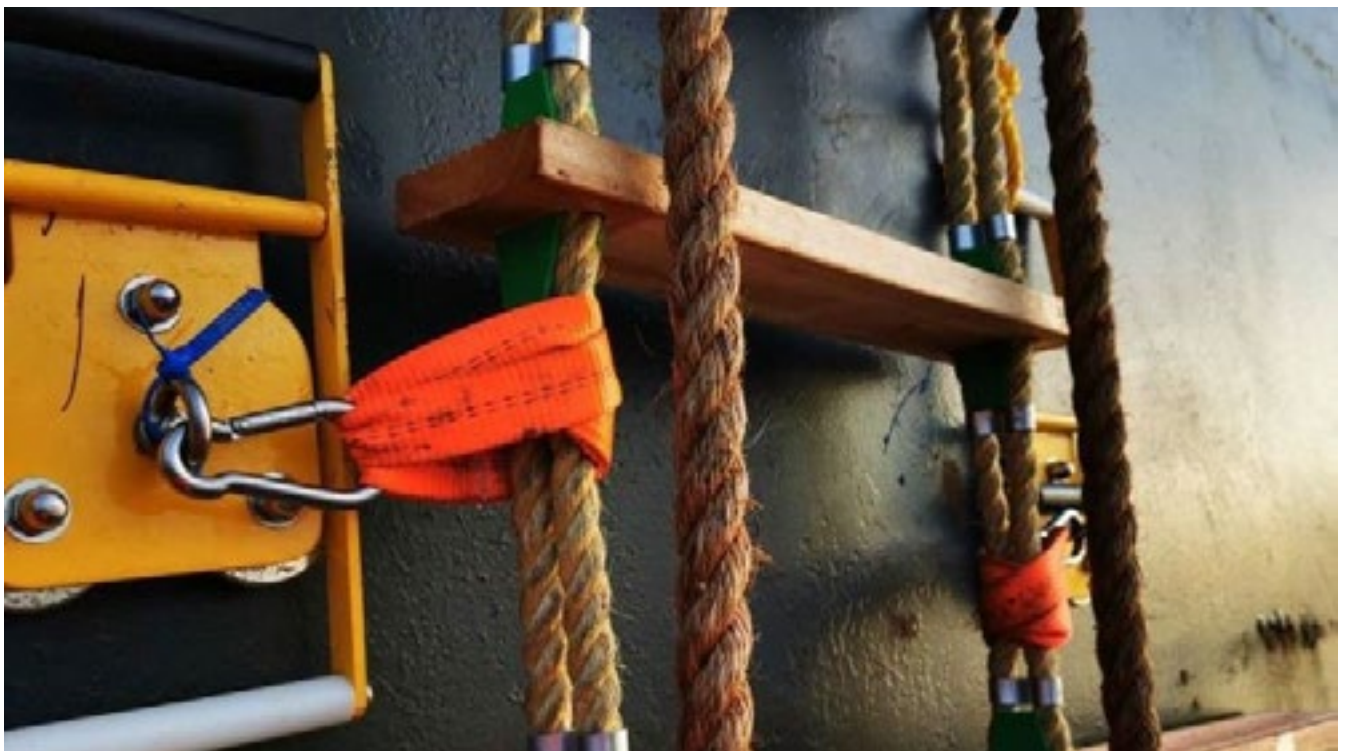
Photo 1: Example of securing both the pilot ladder and accommodation ladders with magnetic pads (Reproduced with permission from Fremantle Ports). Photo credit: AMSA
