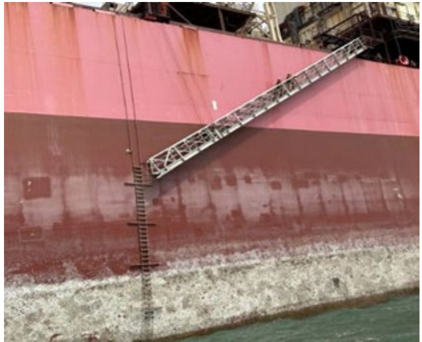
Photo 2: Example of non-compliant combination pilot ladder arrangements. Photo credit: AMSA
