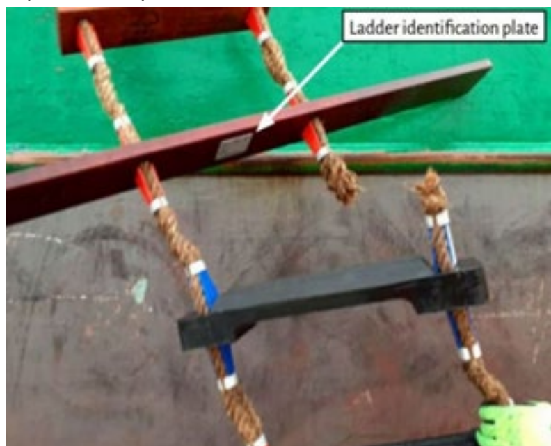
Photo 8: Pilot ladder where side ropes parted when in use (Reproduced with permission of the MAIB). Photo credit: AMSA
