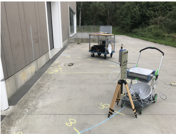
Fig. 2. Measurement setup for fiber cement reflection measurements with a 45^\circ incident angle.
