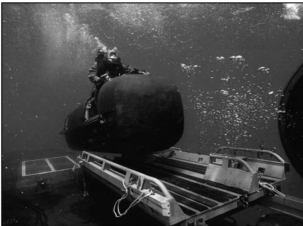
Figure A-2. SEAL Delivery Vehicle Launch from Dry Deck Shelter
