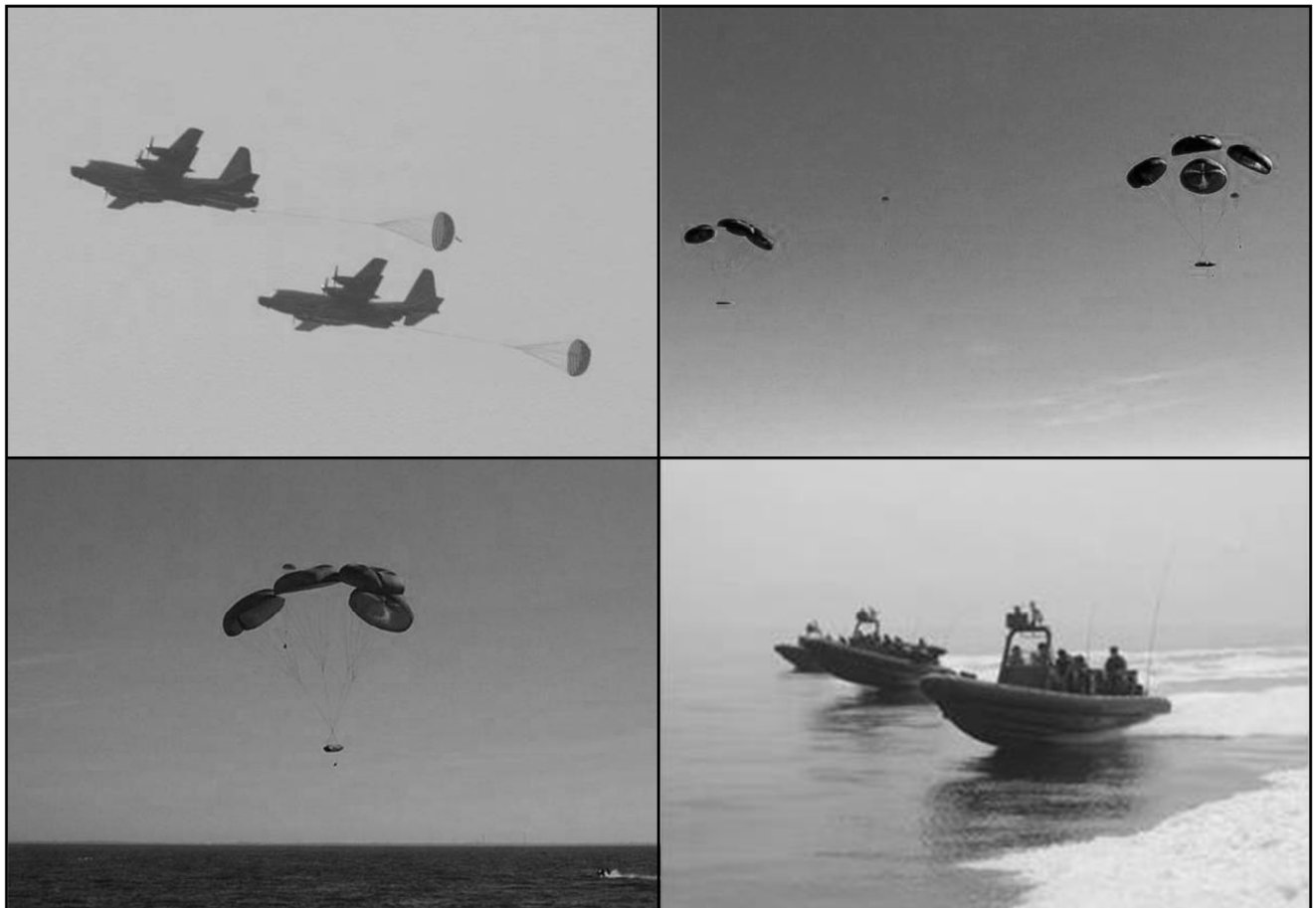
Figure A-8. Maritime Craft Aerial Delivery System
