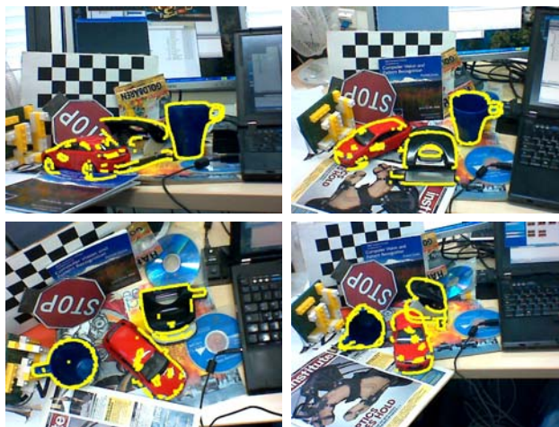
Fig. 1: Our method can detect texture-less 3D objects in real-time under different poses over heavily cluttered background using gradient orientation.
