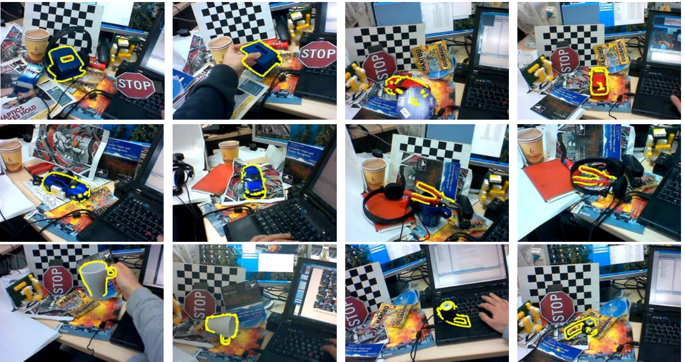
Fig. 15: Different texture-less 3D objects are detected with LINE-2D in real-time under different poses on heavily cluttered background with partial occlusion.
