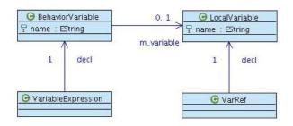
In this schema, classes on the left side belong to the source metamodel while classes on the right side belong to the target metamodel. An important property to be ensured by the transformation is that the diagram commutes: the VarRef image of a VariableExpression refers to the LocalVariable which is the image of BehaviorVariable referenced by the source VariableExpression.
