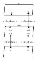
In Fiacre, the processes root\_r and root\_s are composed using interleaving. Their product is synchronized with the glue.
