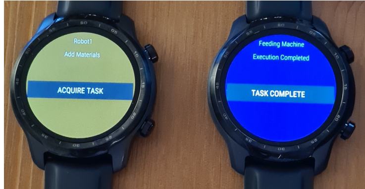
Fig. 2. Photo of the task coordinator app running on two smartwatches. The smartwatch on the right hand side displays a "normal" task. The smartwatch on the left hand side displays an "acquired" task which is currently being performed by the worker.
