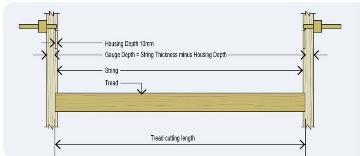
Figure B9: Tread cutting length.
