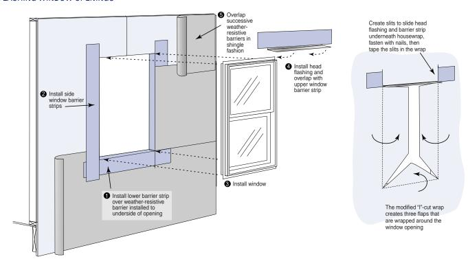
Barrier strips are attached with nails and overlapped with successive barrier strips and weather-resistive barriers in shingle fashion. Do not depend on tapes or glues, as they may fail over time.
