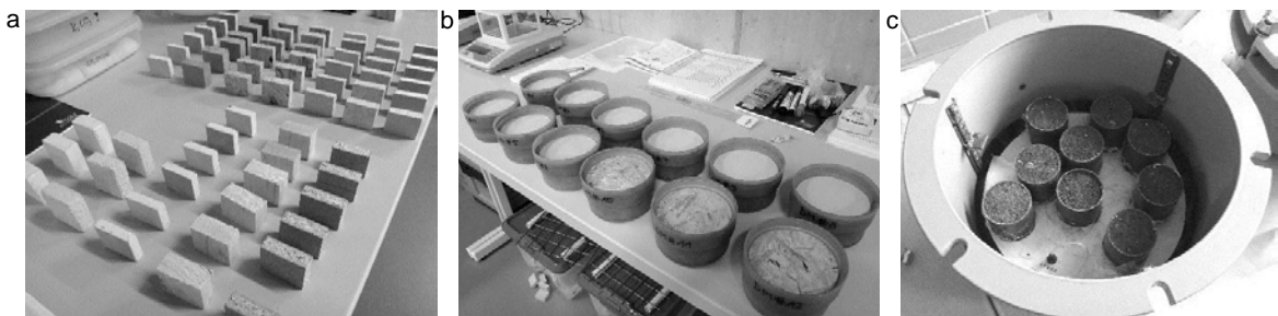
Fig. 4. (a) Samples for sorption; (b) Samples for diffusion; (c) Soil samples for retention.
