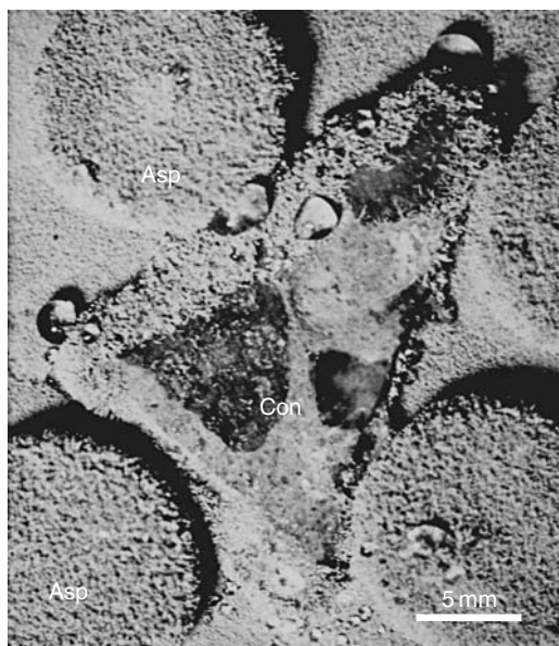
Fig. 5.5. Six-month Petri dish microcosm: Aspergillus flavipes (Asp) colonization of a piece of barrier concrete (Con) inserted into Czapek–Dox agar. Scale bar, 5 mm. Adapted from Fomina et al. (2005c).
