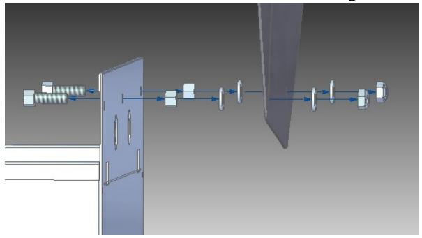
1/4-20 x 3/4" Bolts, 1/4-20 Nuts, Washers, Wall Bracket, Washers, 1/4-20 Locking Nuts
