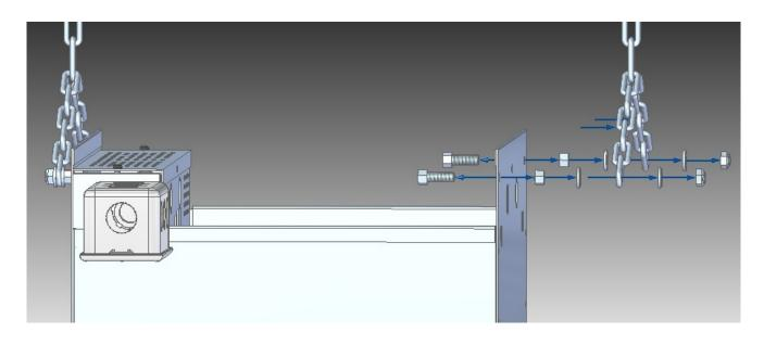
1/4-20 x 3/4" Bolts, 1/4-20 Nuts, Washers, Chains, Washers, 1/4-20 Locking Nuts
