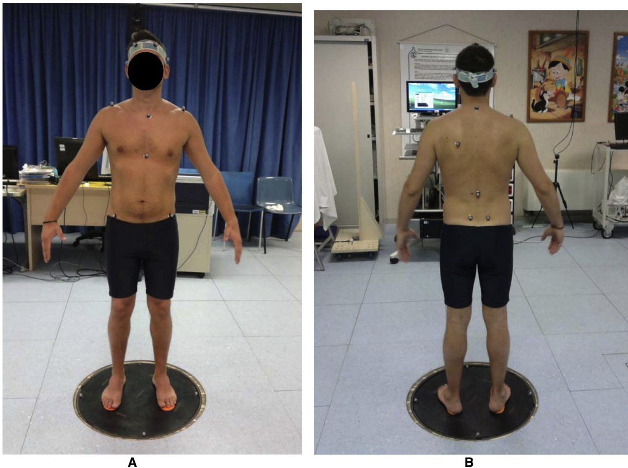
Fig. 2. Front (A) and back view (B) of the experimental setup: moving base, equipped with four retro-reflective markers, and the standing subject, equipped in accordance to the PlugInGait marker set.
