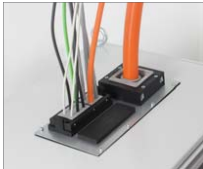
Routing of several cables with and without connectors through a closed enclosure roof via module plates. Cut-out size 314 x 144 mm.
