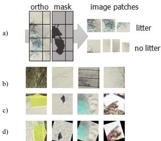
Figure 3. Examples of image samples extracted from the ortho. a) . Ortho and manually defined mask. On the right the resulting image patches, b) litter and c) oversampled litter patches (see section 3.3.2).
