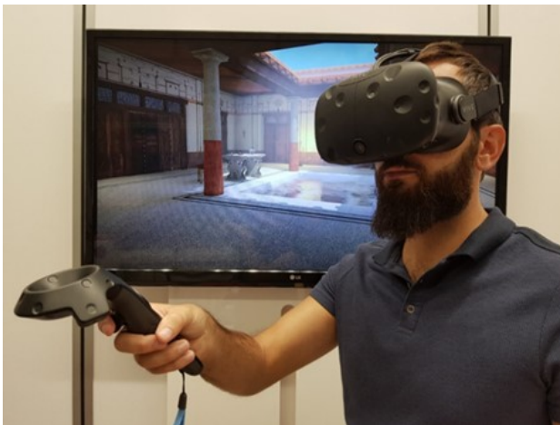
Figure 8. HMD technology for the immersive virtual diving system
