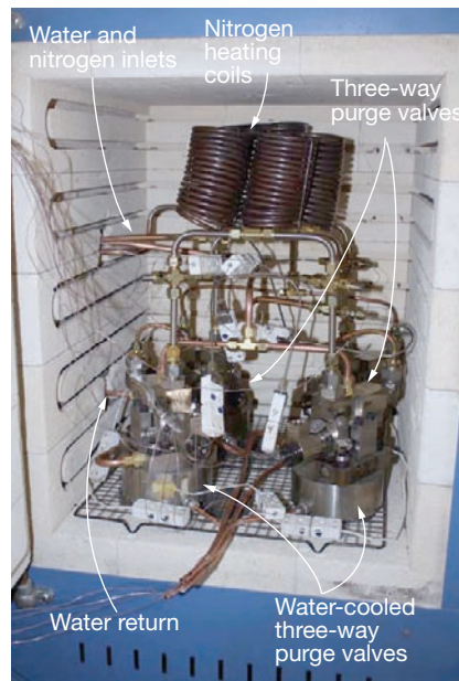
4. Test setup to measure the effectiveness of the water cooling circuit reflects the practical approach to engineering problem-solving championed by JASC President Harvey Jansen. Entire test rig is at left, oven at right
