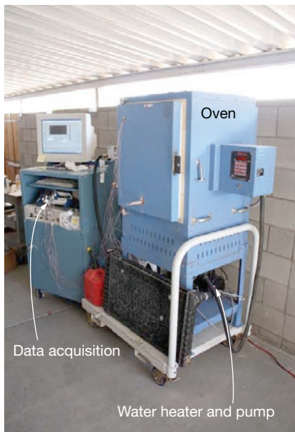
4. Test setup to measure the effectiveness of the water cooling circuit reflects the practical approach to engineering problem-solving championed by JASC President Harvey Jansen. Entire test rig is at left, oven at right
