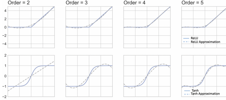
Figure 4: Approximation of ReLU and Tanh activation via the Volterra series formulation
