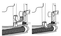
2. Align the tool storage clip with the slot as shown. Slide down the tool storage clip until it is secured into place.
