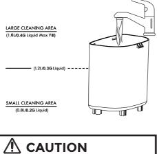
Do not fill with water above 104°F (40°C). Do not exceed filling the clean water tank over the maximum fill line indicated on the clean water tank.
