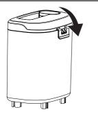
5. Slide the clean water tank back onto the unit. The security latch will automatically secure once the clean water tank is in position. A click will be heard when correctly installed.
