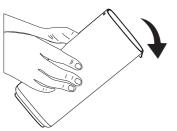
4. Insert the locking tabs into the slots of the dirty water tank first and then secure the dirty water tank cover back into place until a click is heard.
