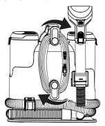
5. Lock power cord plug onto the power cord.
