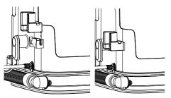
3. Slide the tough stain tool onto the end of the suction hose until it clicks into place.
