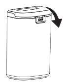
5. Reinstall the dirty water tank back onto the unit. The security latch will automatically secure the dirty water tank in position. A click will be heard when correctly installed.
