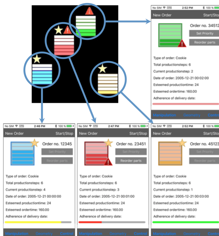
FIGURE 4.19: Touch input applied to the status update view on the smart watch opens a dedicated status report view on the smart phone.
