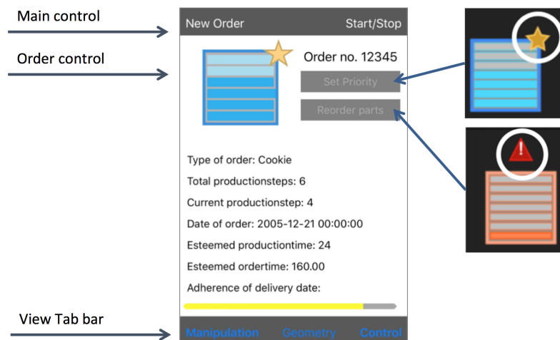
FIGURE 4.20: Status report and dashboard application contains referring custom order glyph, detailed information of the order production, and graphical control elements.
