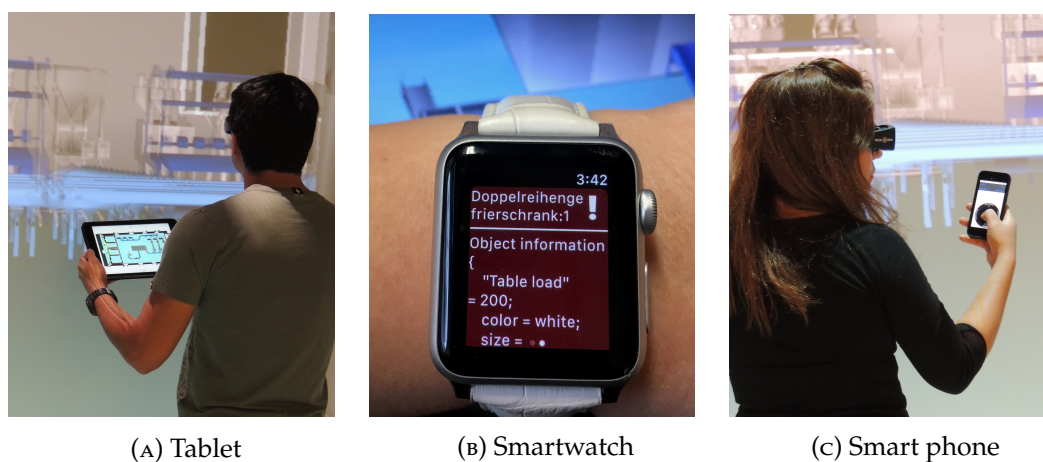
FIGURE 5.13: Integrated smart devices acting as input and secondary output-devices scaling from smartwatch to tablet computers
