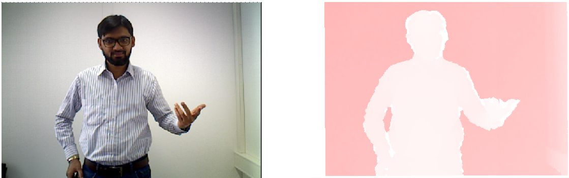
Figure C.1: Colour and depth stream of the scene from OpenNI software.
