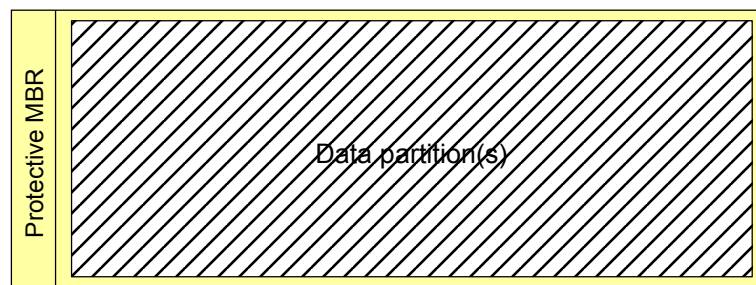
Figure 1-17 General GPT disk structure
