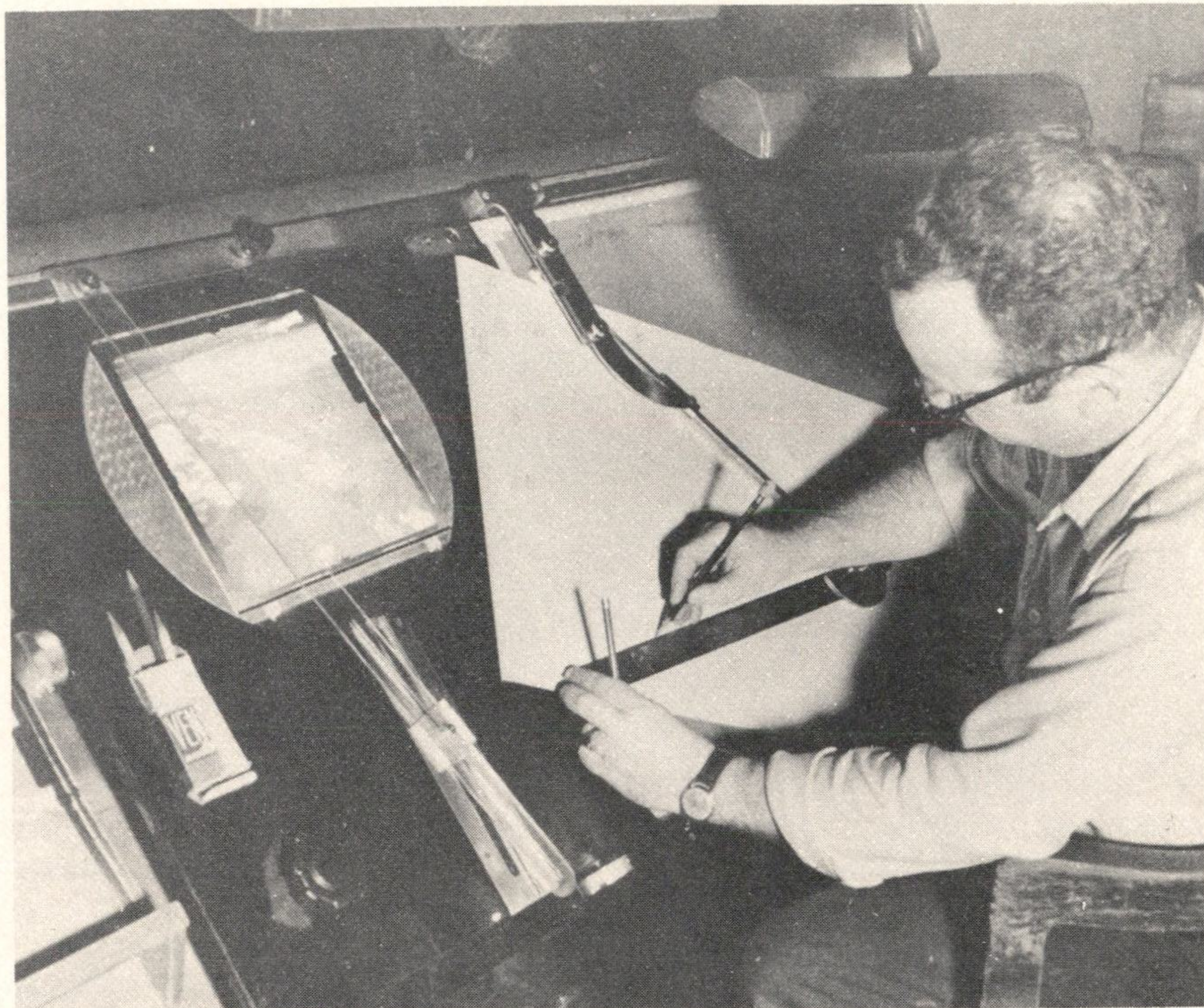
Radial line plotter makes a single paper template from three simultaneous trimet- rogon exposures.
