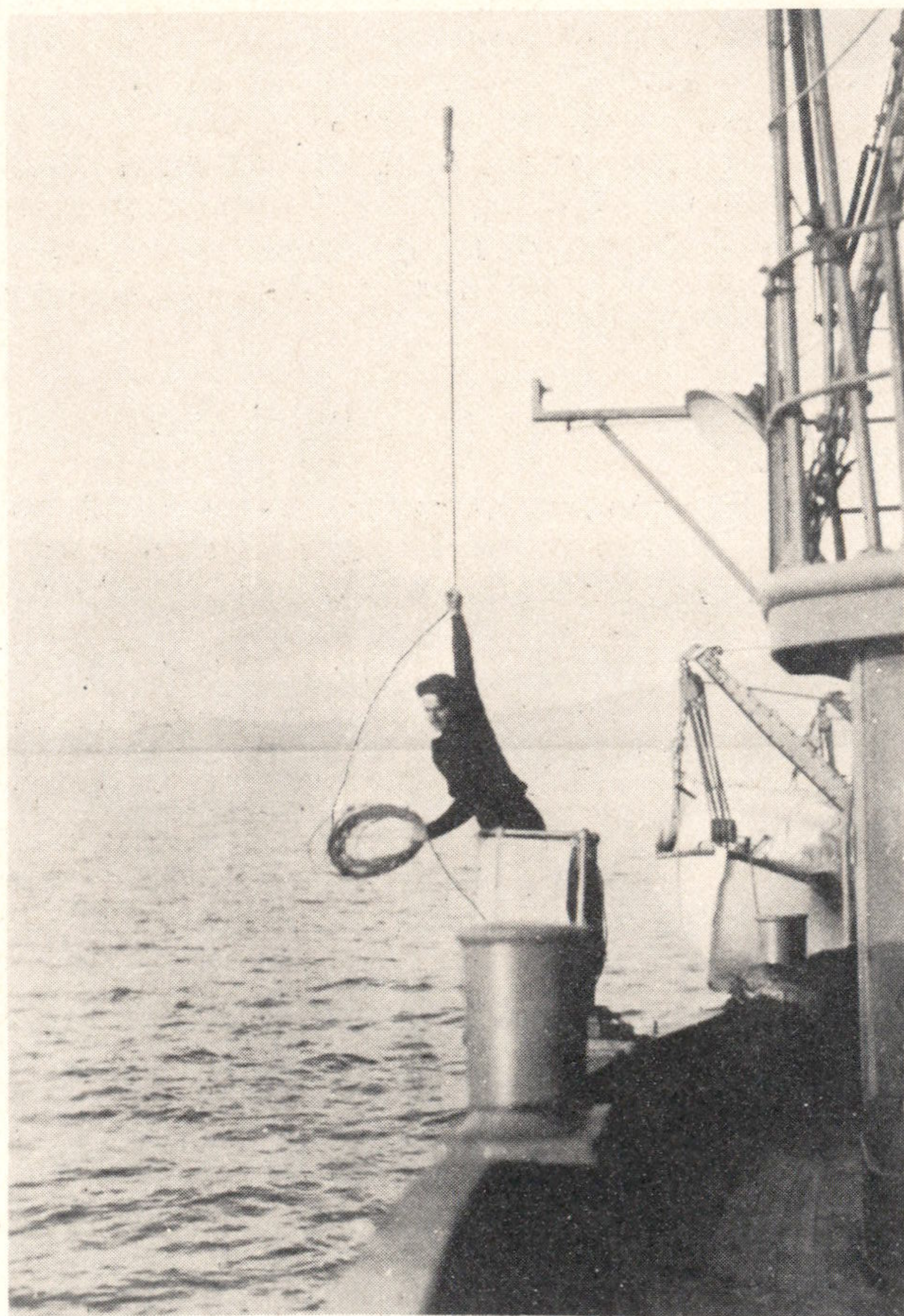
Sounding with the hand lead was the common method of doing hydrography in the Islands.
