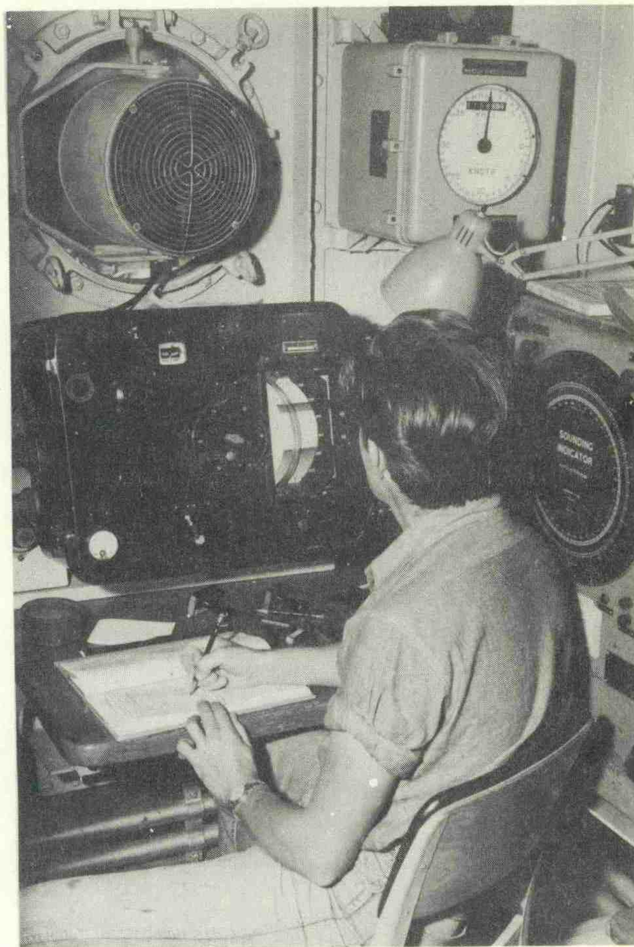
Type 808 portable graphic-recorder revolutionized sounding methods.
