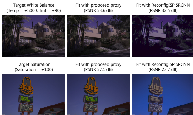
Fig. 7. Proxy Comparison of Proposed and ReconfigISP [2021] SRCNN proxy architecture. The “one-size-fits-all” architecture used by ReconfigISP is unable to accurately model the operations found in complex commercial pipelines such as ACR. Here, we show that our proposed architectures act as better proxies for the individual modules.
