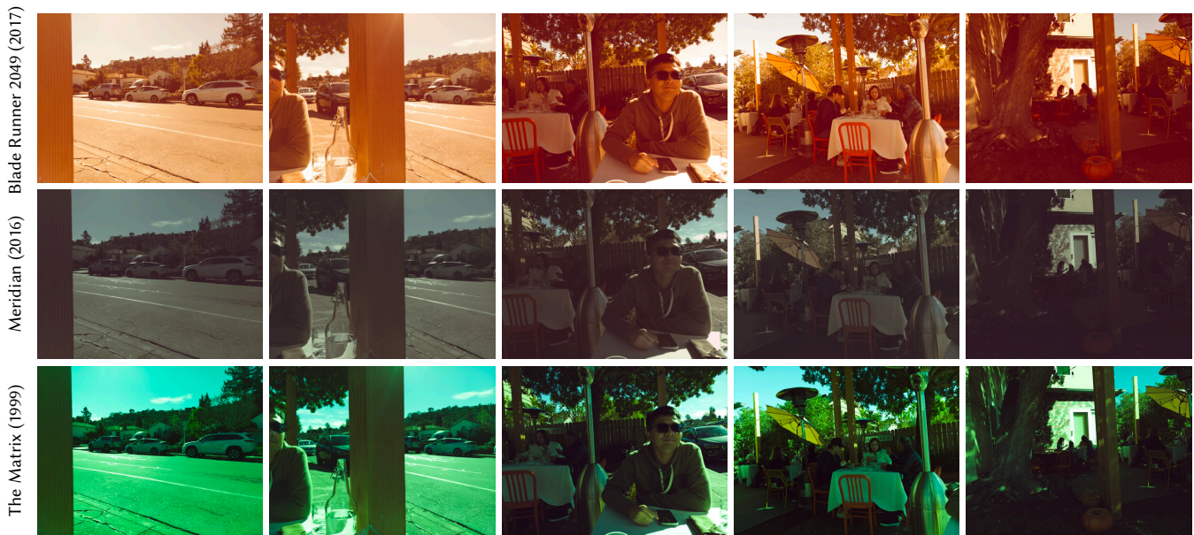
Fig. 11. Video Style Transfer. We apply the three movie styles from Figure 10 to a few raw videos of our own. Our approach of predicting slider values makes the style transfer temporally consistent throughout the sequence even when it contains large changes in dynamic range (e.g., from sunlight to shade). See the Supplementary Video for all video results.
