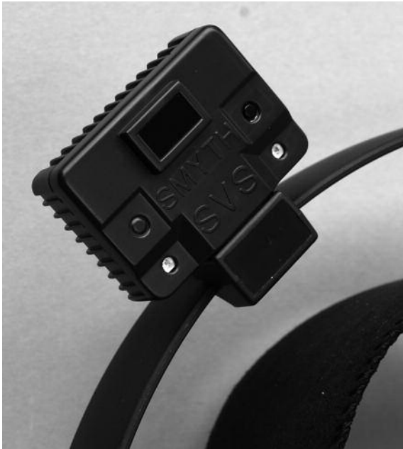
Photo 2 The head angle transmitter on top of the headphone band.
