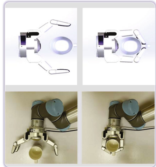
Fig. 10 Grasping procedures with a different mug configuration by the nominal models and the practical applications
