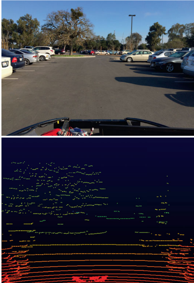
Fig. 5.3 Above: a driving scene with parked cars. Below: the view from a laser scanner
