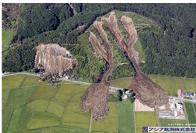
Fig. 5 Most landslides are shallow, several meters deep-seated, and are mostly classified as planar types (left) and spoon types (right)
