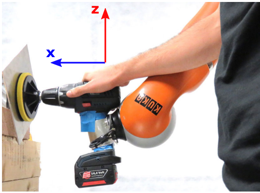
Fig. 2 Experimental setup for collaborative surface polishing. The arrows show the robot base frame
