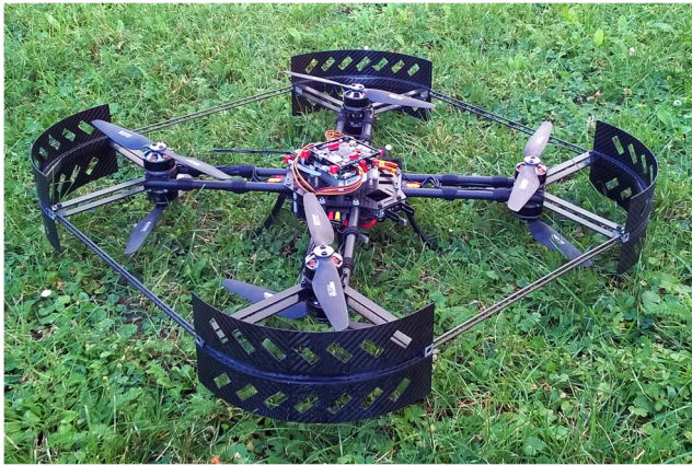
Fig. 1 The Falcon V5 coaxial quadrotor developed at the Institute of Control, Robotics and Information Engineering of Poznan University of Technology
