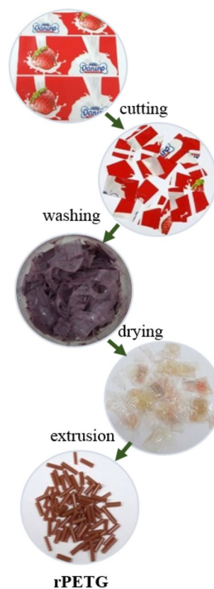
Fig. 1 Mechanical recycling process of PETG, starting from printed waste foils and ending with regranulate pellets
