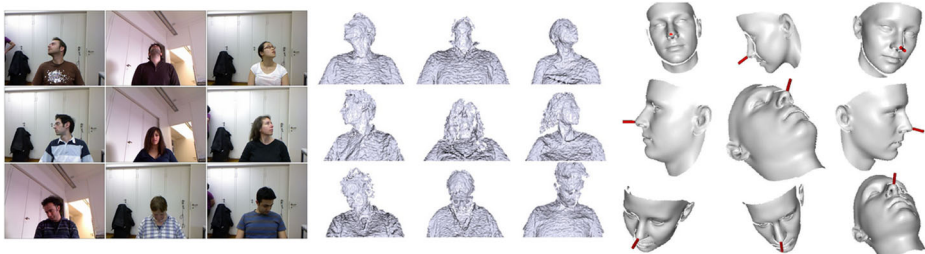
Fig. 9 From left to right: RGB images, depth images and depth images with annotations from Biwi Kinect Head Pose Dataset [25]
