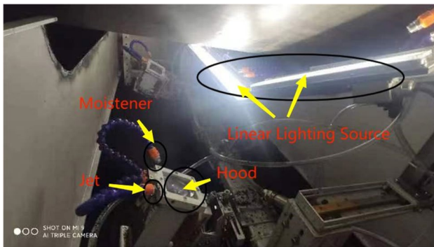
Fig. 12 The installation diagram of camera and linear light source
