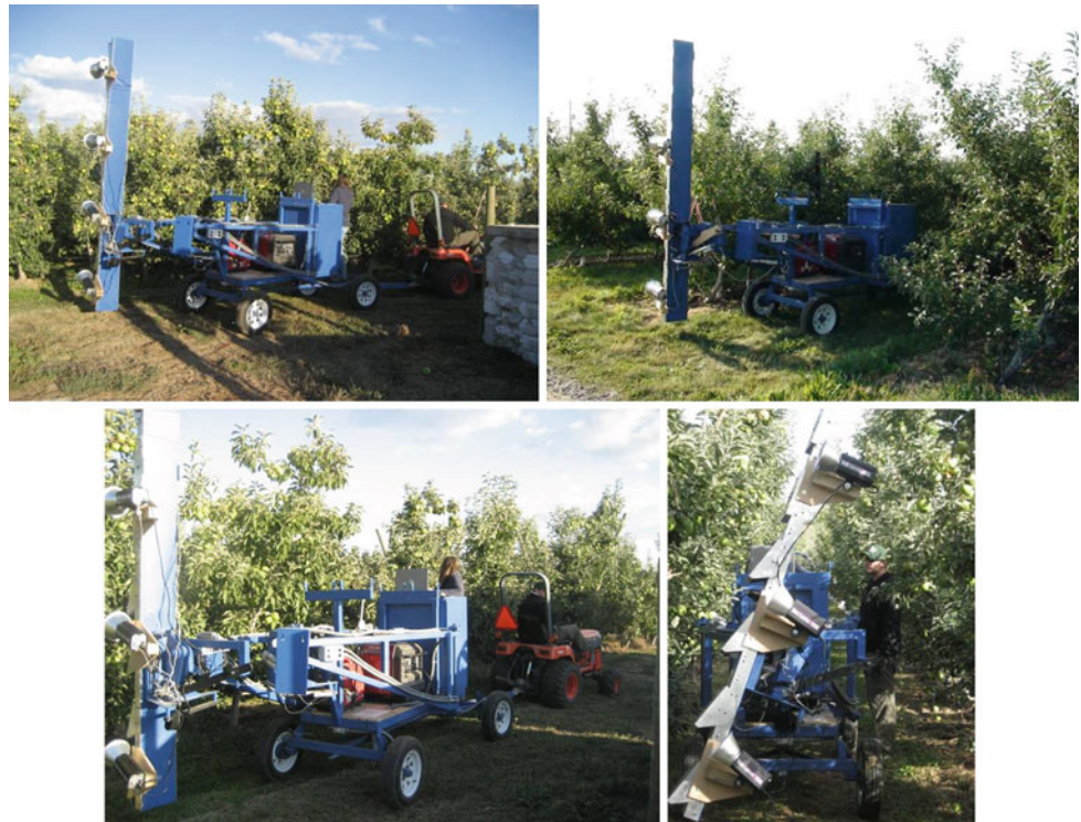
Fig. 16 The Scout in the field. The mast, which houses the cameras and flash units, is mounted on an arm that can be moved to adjust the mast position relative to the trees
