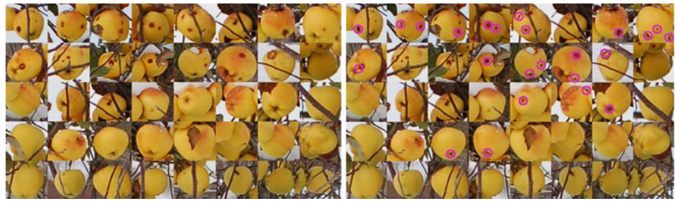
Fig. 12 Left Original images of apples. Right The regions detected as IFW-damaged
