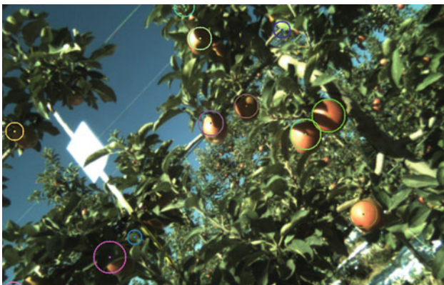
Fig. 20 Representative image showing apples identified by the (back-end) software
