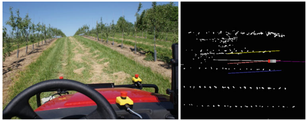
Fig. 6 Sloped terrain (curving uphill) brings the ground itself into view of the lasers. This causes the row detector to produce a poor result. A low-pass filter on the row detection dampens this effect
