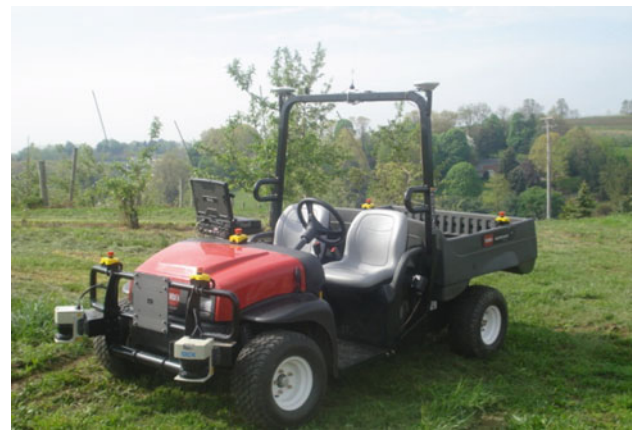
Fig. 2 First autonomous prime mover, based on a Toro MDE eWorkman vehicle
