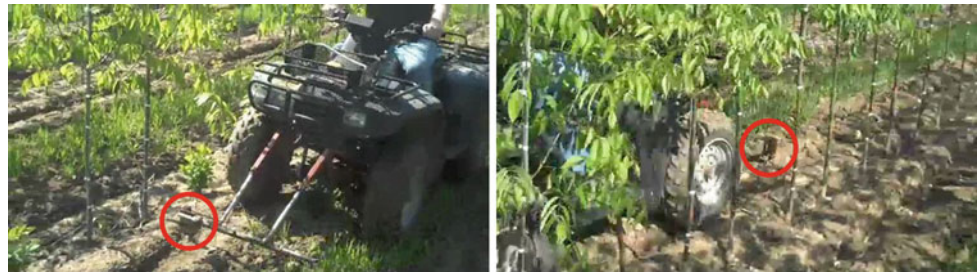
Fig. 22 Rigid mount and camera (inside circle) on ATV used to collect imagery to assess the challenges to be addressed by the automated caliper and counter devices
