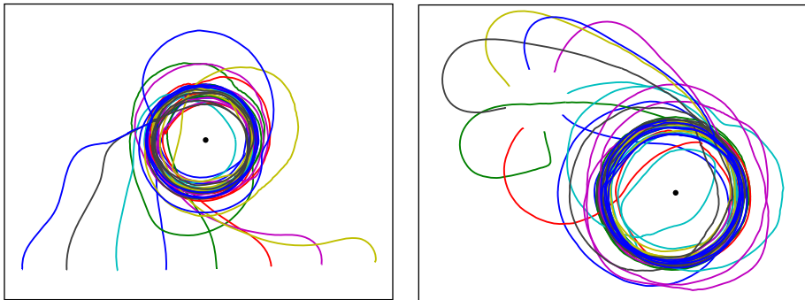
Fig. 8 Full extracted trajectories of the eight robots through the duration of experiments, for initial conditions 1 ( left ) and 10 ( right )
