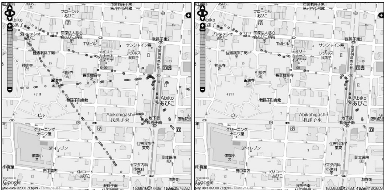
Fig. 6 Quality filtering result in the OpenLayers interface
