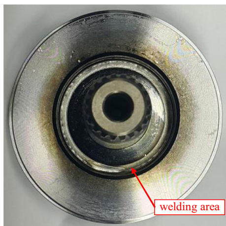
Fig. 1 Top view of the welded engine transmission. The shape of the welding area is circular
