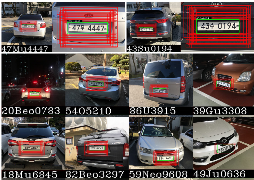
Fig. 6. Examples of license plate recognition and detection on the test images.
