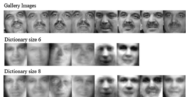
Fig. 3 Examples of the K-SVD learned dictionaries for one subject in LFW database. The images in each sub-figure contain a group of gallery or probe images from the same subject. The bottom of the two images in each sub-figure are dictionaries which are learned from the top images. These K-SVD learned dictionaries have different sizes
