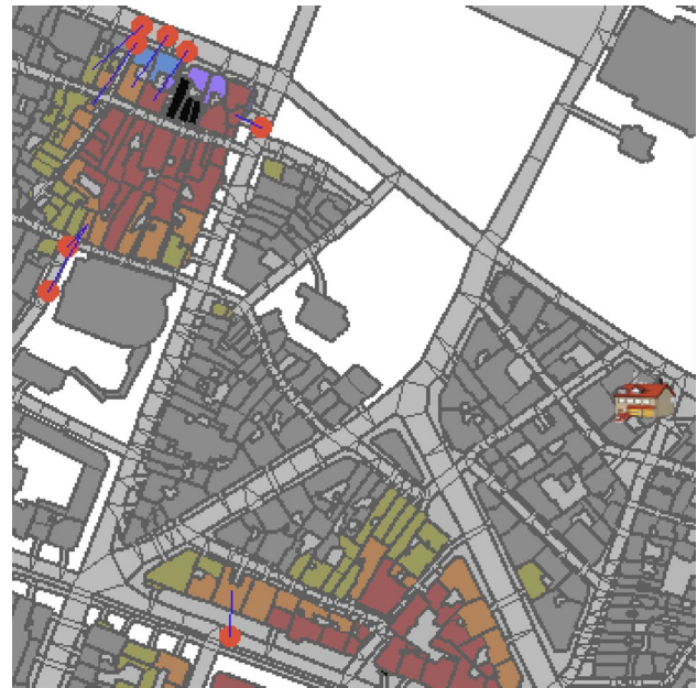
Fig. 2 Detail of an example problem on the Paris map. The red dots are fire brigades and the blue lines are their water jets. The colour of the buildings reflects their status: grey means no damage; yellow to red means on fire; blue to purple means that the fire has been extinguished, and black means that the building is burnt. The darker the colour, the greater the damage. On the centre-right is a fire station, to which the fire brigades return to refill
